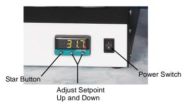
9 To heat the reagent flask, turn on the power switch on the face of the distillation chamber. To enter a setpoint (i.e., the desired heater temperature), hold in the 'star button', then while holding the star button, press the Up arrow to increase and the Down arrow to decrease the setpoint temperature. The setpoint temperature appears in the display anytime that the star button is pressed. When no keys are pressed, the sensed temperature in the distillation chamber is displayed.
