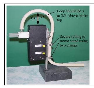
For the stirrer to run properly, it's important that the vacuum tubing does not restrict rotation. Secure the supplied length of vacuum tubing to the post of the stirrer stand as shown, making sure that the connection is tight enough that the tube will not move, but not so tight as to restrict the vacuum. The vacuum tube should form a 3 to 3.5" loop above the stirrer unit as shown.
