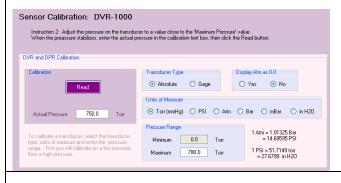
Now remove the vacuum source and allows the vacuum transducer to set at atmospheric pressure. Enter the current barometric pressure in the box titled "Actual Pressure" and click the Read button. Remember, pressures must be entered as Absolute pressure, so enter the actual barometric pressure, which is probably not 14.69 psi (i.e., exactly 1 atmosphere).
