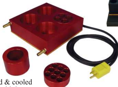
Two temperature zone block for reagent and reaction vials
