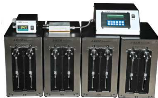
Microfluidic reaction system delivers 24 reagents to a heated reactor. PC control automates 1000 reaction combinations
