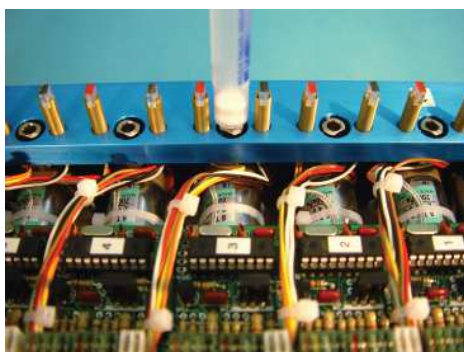
Inside of a SPE controller showing flow rate control and solvent front optical detector electronics
