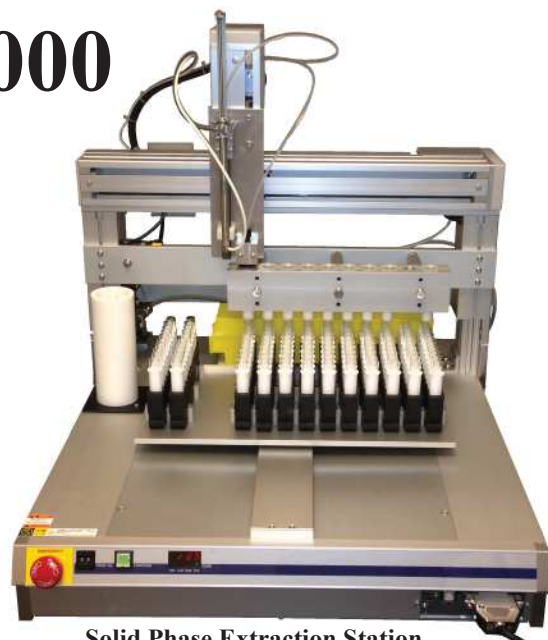
Solid Phase Extraction Station Runs 10-step elution program
