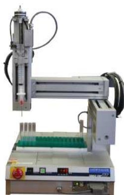
Smart Fraction Collector Switches between titer plates and 50 ml tubes under program control
