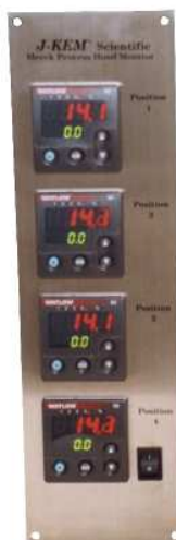
Four position temperature controller designed to fit on the front face of a research hood
