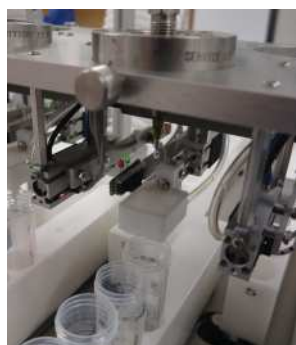
Noninvasively measures flow rate by counting precision formed drops
