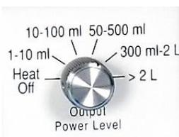
The power control computer is always set to the **Volume** of solution being heated, not the size of the flask or heater.
