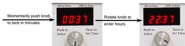
**Step 4.** When the desired time is displayed, hold in the timer knob for 1 second to enter the time and start the timer. When the timer starts, the LED under the label “ON at Zero” lights. This indicates that power to the heater will turn ON when the timer counts down to zero.
