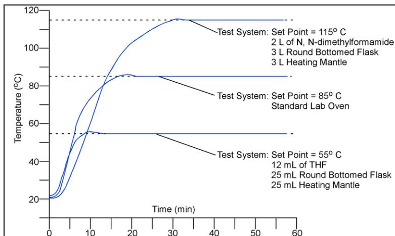
When the power control computer is set to the correct power level, your controller can regulate virtually any heater to  $\pm 0.1^\circ\text{C}$  with less than  $1^\circ\text{C}$  overshoot on initial warming.
