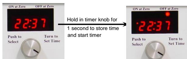
At any time, the timer program can be aborted by holding in the timer knob for 1 second. When this is done, the display changes to toFF. To turn on heating, push the timer knob twice until the display reads On.
