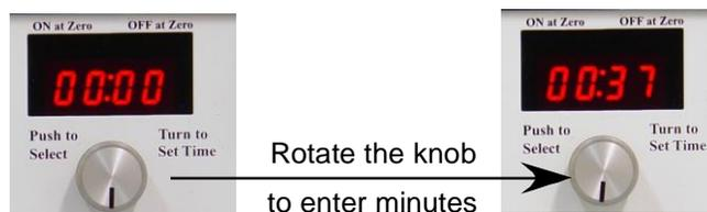
**Step 3.** To change the number of hours in the display, momentarily press the timer knob (1/4 second) and the hours digits begin to blink. To increase the number of hours, rotate the timer knob to the right. To decrease the number of hours, rotate the timer knob to the left.
