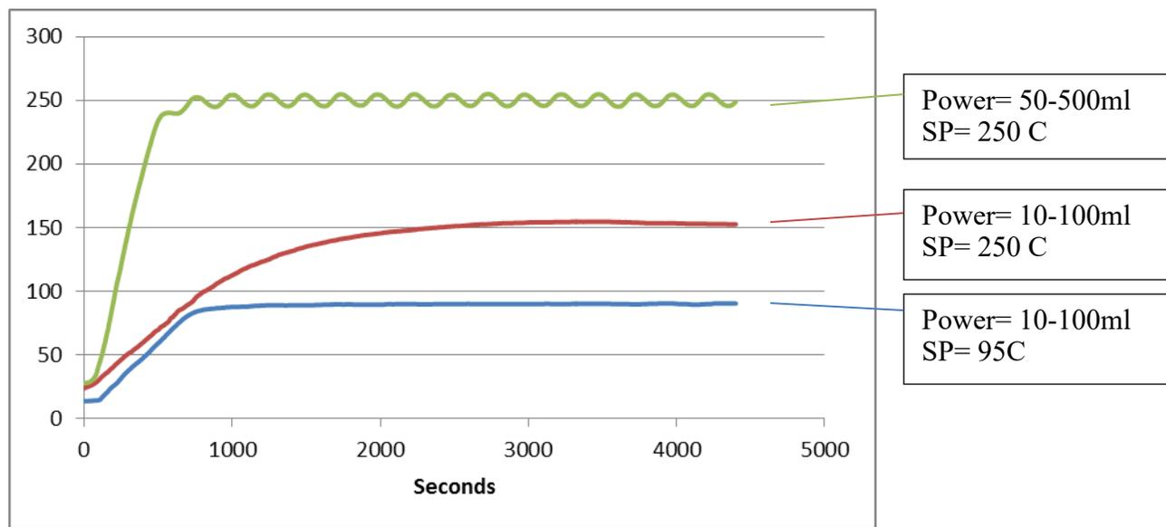
The bottom plot uses the standard set of PID values that results in stable temperature control at 95 C.
