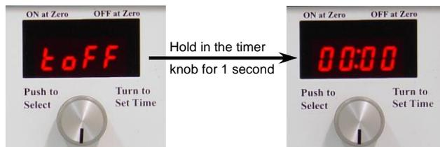
**Step 2.** To increase the number of minutes, rotate the timer knob to the right. To decrease the number of minutes, rotate the timer knob to the left.
