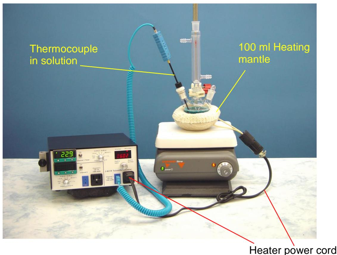
4. Enter the temperature that you want to heat the reaction to (i.e., the Setpoint) into the digital meter.
