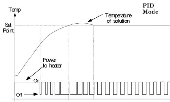
In PID mode the controller monitors the shape of the heating curve during initial warm up and decreases power to the heater before the set point is reached so that the solution reaches the set point with minimal overshoot. [Notice that the heater turns off for varying periods of time before the set point temperature is reached]. The second feature of PID mode is that it adjusts the percent of time the heater is on so that the set
