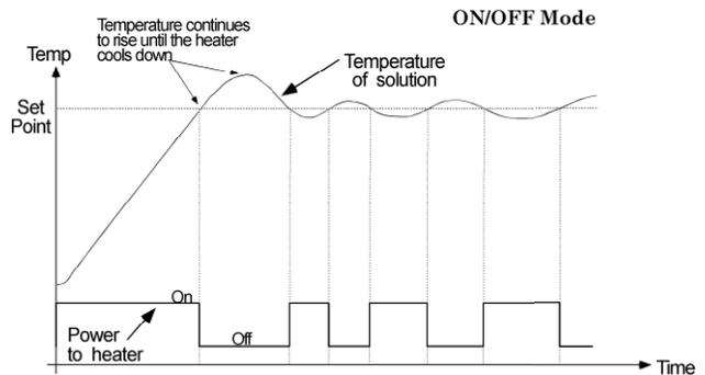
continues to rise. This method works well for heaters that transfer heat rapidly (such as heat lamps), it's acceptable for heaters such as heating mantles ( $\approx 5^\circ$  overshoot), but it's terrible for heaters that transfer heat slowly (vacuum ovens, heating blocks, etc.).
