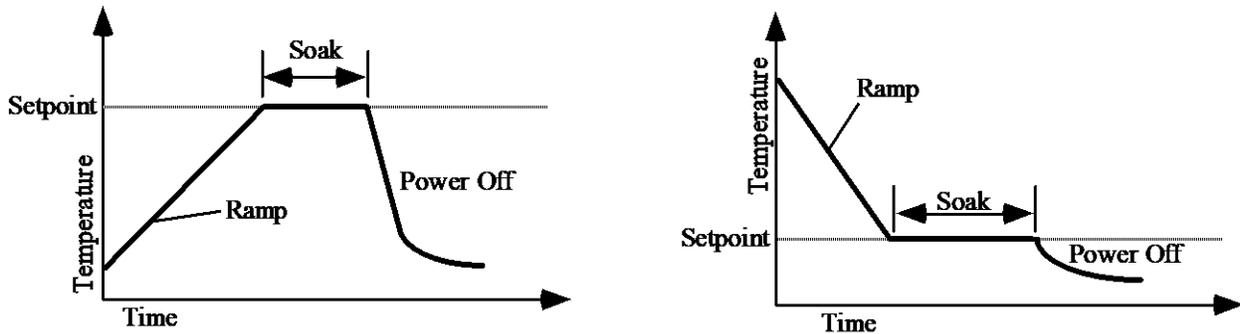
The controller is shipped with the Ramp-to-Setpoint feature OFF, the user must specifically turn Ramp-to-Setpoint ON. When Ramp-to-Setpoint is OFF, the controller heats to the entered setpoint at the fastest rate possible. When Ramp-to-Setpoint is ON, the controller heats at the user entered ramp rate. The Ramp-to-Setpoint feature and its associated parameters are turned on and set in the controller's programming mode. The parameters of importance are:
