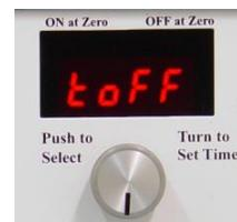
**Step 1.** When the timer displays “toFF”, holding in the timer knob causes the display to change to a clock showing 00 : 00. The left 2 digits are hours and the right 2 digits are minutes. The minutes digits are blinking which indicates that their value can be changed.
