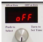
To turn power On to the heater, briefly push in on the round timer knob and the display changes to ON to show that power to the heater is ON. For complete instructions on the user of the timer see the section titled *Timer Controls*.
