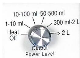
The power control computer is always set to the **Volume** of solution being heated, not the size of the flask or heater.
