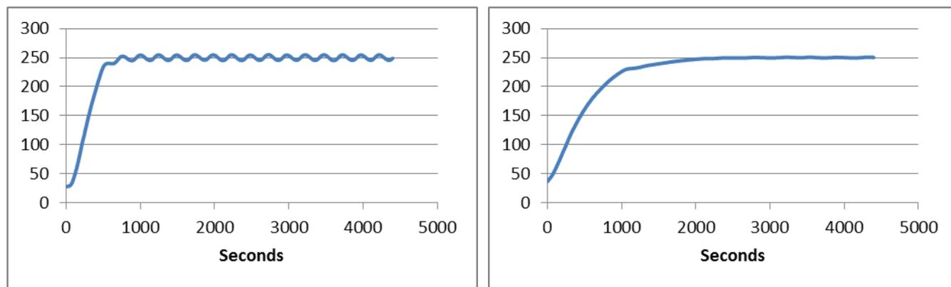
The answer to remove the oscillation shown in the chart on the left is to autotune the controller, which results in the temperature profile shown on the right.
