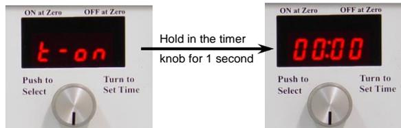
**Step 2.** To increase the number of minutes, rotate the timer knob to the right. To decrease the number of minutes, rotate the timer knob to the left.
