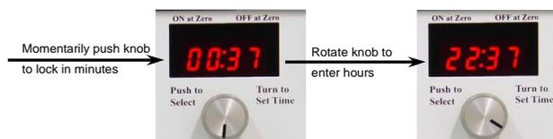
**Step 4.** When the desired time is displayed, hold in the timer knob for 1 second to enter the time and start the timer. When the timer starts, the LED under the label “OFF at Zero” lights. This indicates that power to the heater will turn OFF when the timer counts down to zero.
