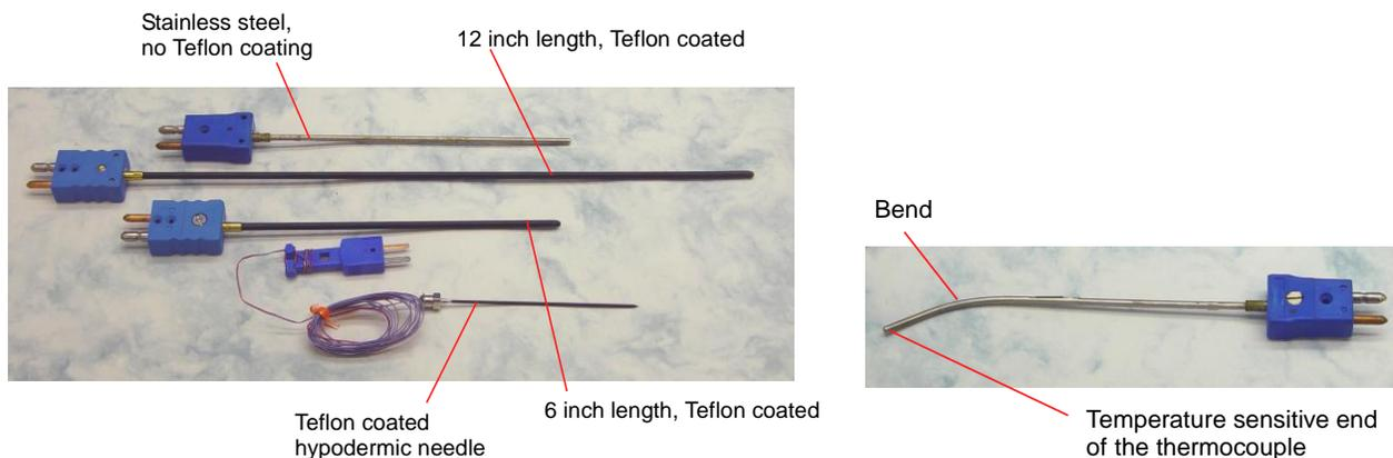
When a thermocouple is placed in solution, often it is desirable to bend the thermocouple slightly so that more of the tip extends into the solution. It does not hurt a thermocouple to be bent slightly. The temperature sensitive portion of a thermocouple is the first ¼” of the tip. It’s good for the first ½” to be in solution, but the first ¼” must be in solution to read the temperature correctly.
