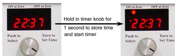
At any time, the timer program can be aborted by holding in the timer knob for 1 second. When this is done, the display changes to t-on. To turn on heating, push the timer knob until the display reads On.
