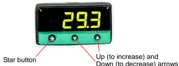
5. Set the correct Power Control Level. Your J-KEM controller has a built in Power Control Computer (PCC) that precisely regulates power to the heater. For the computer to work correctly, it must know the volume of solution that is being heated. It's important to understand that the PCC is set to the **Volume** of solution being heated, not the size of the heater or the size of the flask.
