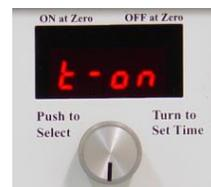
**Step 1.** When the timer displays “t-on”, holding the timer knob in for 1 second causes the display to change to a clock that shows 00 : 00. The left 2 digits are hours and the right 2 digits are minutes. The minutes digits are blinking which indicates that their value can be changed.
