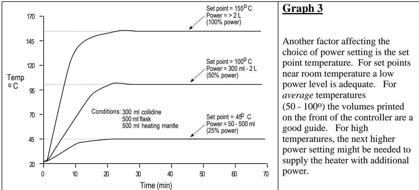
The power reduction circuit limits the total amount of power delivered to the heater. In this sense it works like a variac and can be used like one. If the heater isn't getting enough power, turn the power level up one notch, if it's getting too much power, turn it down.
