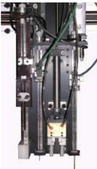
Sample of J-KEM's Z-axis plate with two septum penetrating needles, vial gripper, and septum penetrating analytical syringe.
